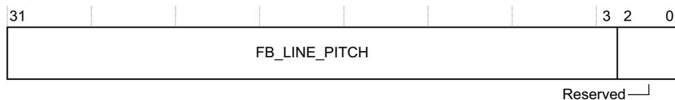
**Figure 3-44** Frame Buffer Line Count Pitch bit assignments
