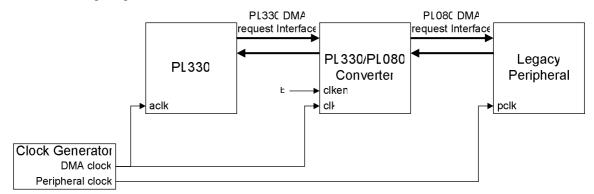
Note that the PL080 DMA request interface is an asynchronous interface. Therefore the integration method illustrated above will work correctly as long as the frequency of the Peripheral clock is less than or equal to the DMA clock.
