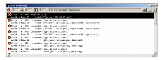
The code pane of the window opens the relevant source file and an arrow highlights the line of code associated with the first error message. There is something wrong with the code; a close bracket is missing. The line should read:
