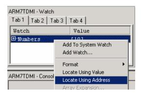
A memory window opens with the contents of the first element of the array highlighted.
