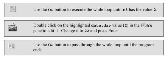
Note how the value entered in variable watch pane affects the value in the register r3, the corresponding entry in the memory window and the program output.
