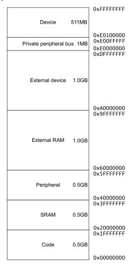
The processor reserves regions of the PPB address range for core peripheral registers, see *About the Cortex-M0 processor and core peripherals* on page 1-2.
