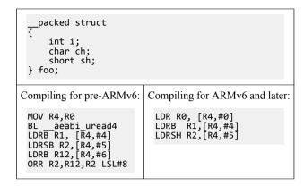
Code compiled for ARMv6 only runs correctly if you enable unaligned data access support on your processor. You can control alignment by using the U and the A bits in the CP15 register c1, or by tying the UBITINIT input to the processor HIGH.
