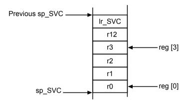
Figure 5-5 Accessing the Supervisor mode stack
