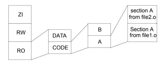
Figure 2-3 Linker placement rules
