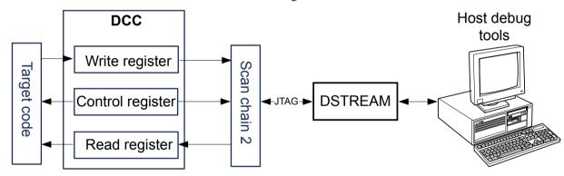
Figure 6-1 DCC communication between target and host debug tools
