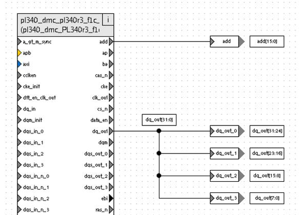
Figure 6-4 Multiple bit-slice connections
