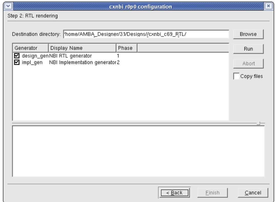
**Figure 4-3 Example RTL generation window for AMBA 4 components**
