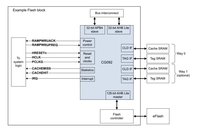
Figure 2-1 Example eFlash implementation
