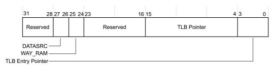
Figure 3-5 SMMU\_DBGRPTRTCU register bit assignments
