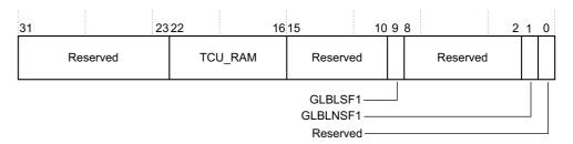
Figure 3-9 SMMU\_ITOP\_GLBL register bit assignments
