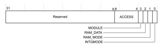
Figure 3-7 SMMU\_ITCTRL register bit assignments
