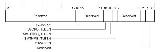
Figure 3-3 SMMU\_sACR Register bit assignments
