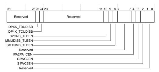
Figure 3-2 SMMU\_ACR Register bit assignments
