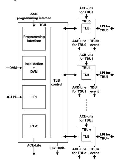
Figure 2-1 MMU-500 block diagram
