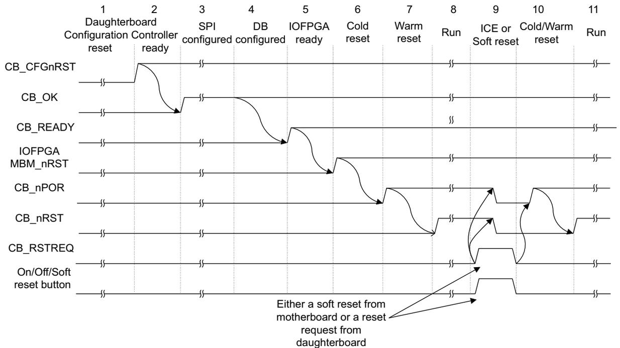
Figure 2-7 CoreTile Express A15x2 A7x3 daughterboard configuration and reset timing cycle
