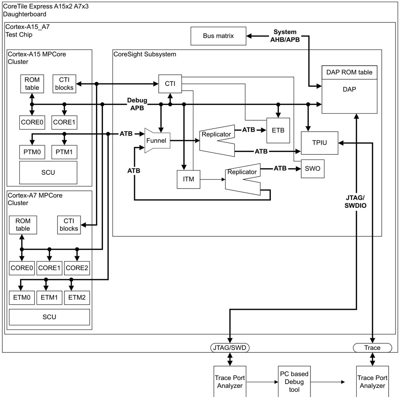
**Figure 2-16 CoreTile Express A15x2 A7x3 CoreSight and trace**
