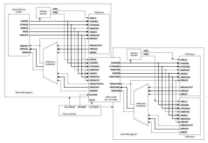
Figure 5-23 Using AHB to AHB sync-up bridge
