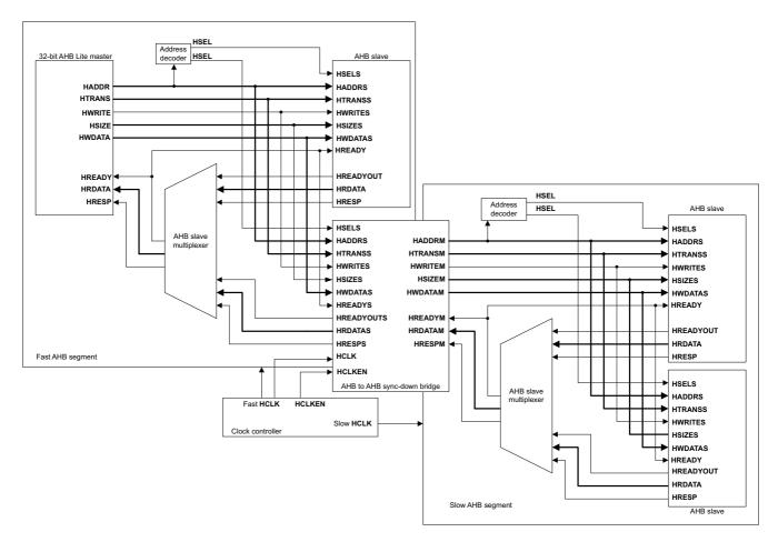
Figure 5-19 Using AHB to AHB sync-down bridge
