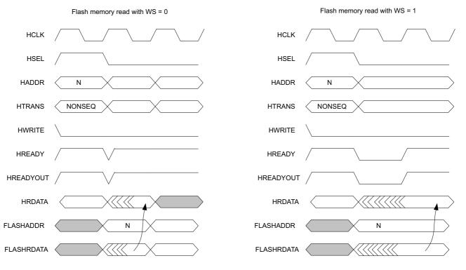
Figure 3-14 AHB to flash read access timing
