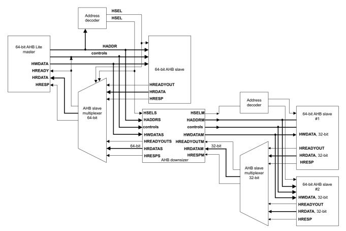
Figure 5-10 Using AHB downsizer, multiple connection
