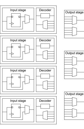
Figure 5-2 Example bus matrix design configuration
