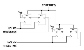
Figure 5-14 Example reset synchronizer
