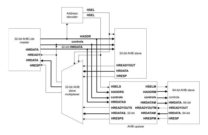
Note: The controls included are HTRANS, HWRITE, HSIZE, HPROT, and HBURST.
