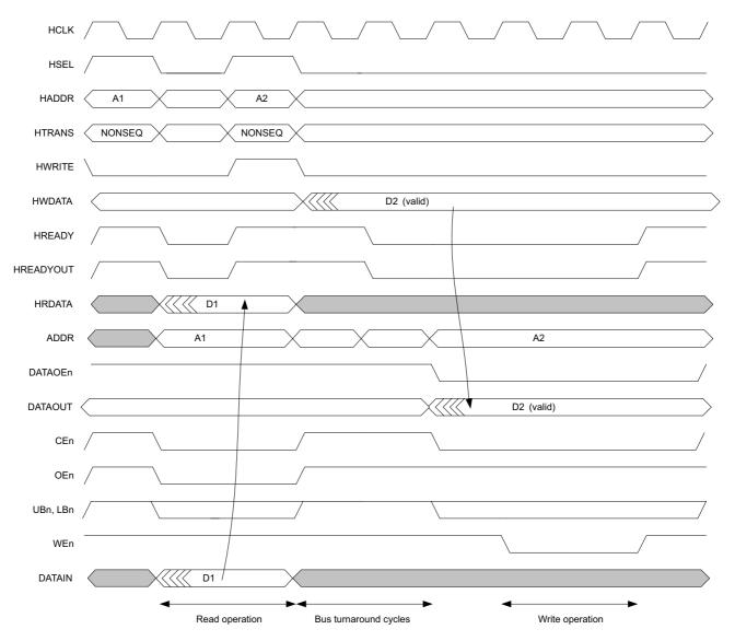
Figure 3-19 External SRAM interface timing 2
