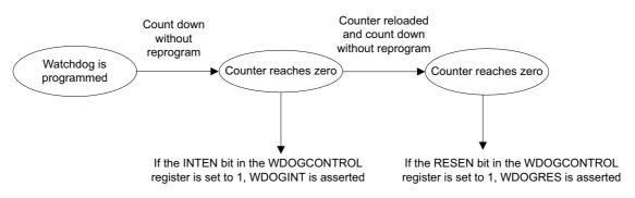
Figure 4-15 Watchdog operation flow diagram
