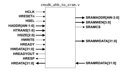
Figure 3-10 AHB to SRAM interface module
