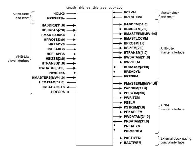
Figure 5-13 AHB to AHB and APB asynchronous bridge
