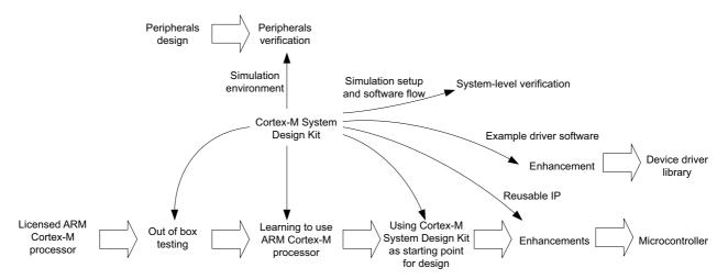
Figure 1-1 Cortex-M System Design Kit usage in various stages of a design process
