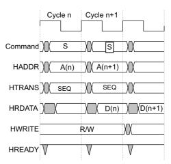
Figure 7-7 Sequential command timing
