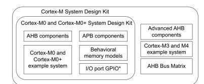
\* For use with the Cortex-M0+ directly, or as a subcomponent within AHB GPIO module.
