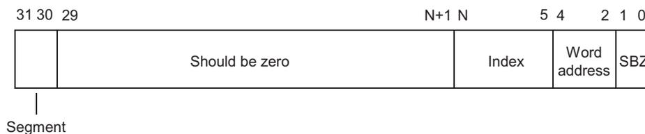
**Figure 2-5 Register 15, Index and segment format**
