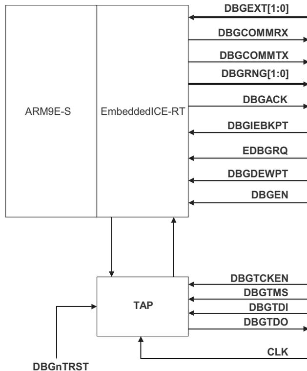
**Figure 9-10** The ARM9E-S, TAP controller, and EmbeddedICE-RT
