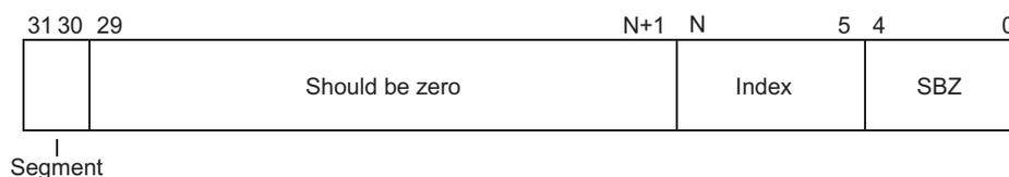
**Figure 2-2 Register 7, Index and segment format**
