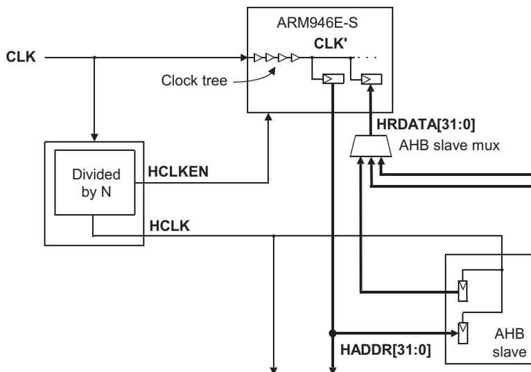
**Figure 6-8 ARM946E-S CLK to AHB HCLK sampling**
