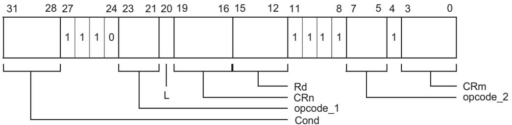
**Figure 2-1 CP15 MRC and MCR bit pattern**
