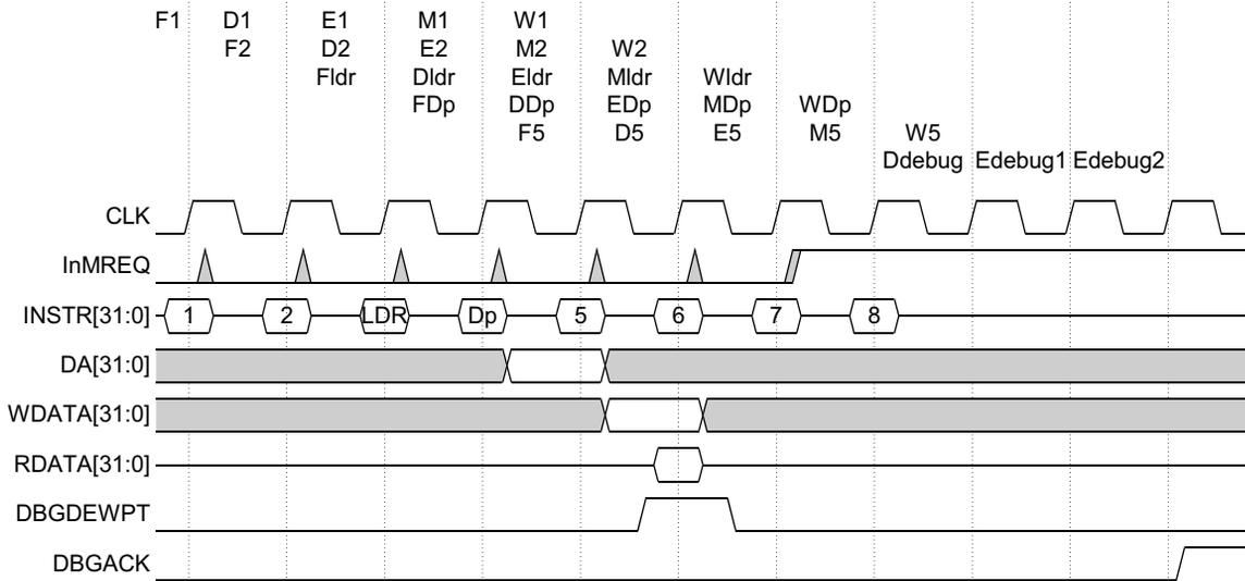
**Figure 9-8 Watchpoint entry with data processing instruction**
