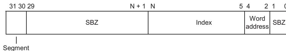
**Figure 9-6 Cache Index Register format**
