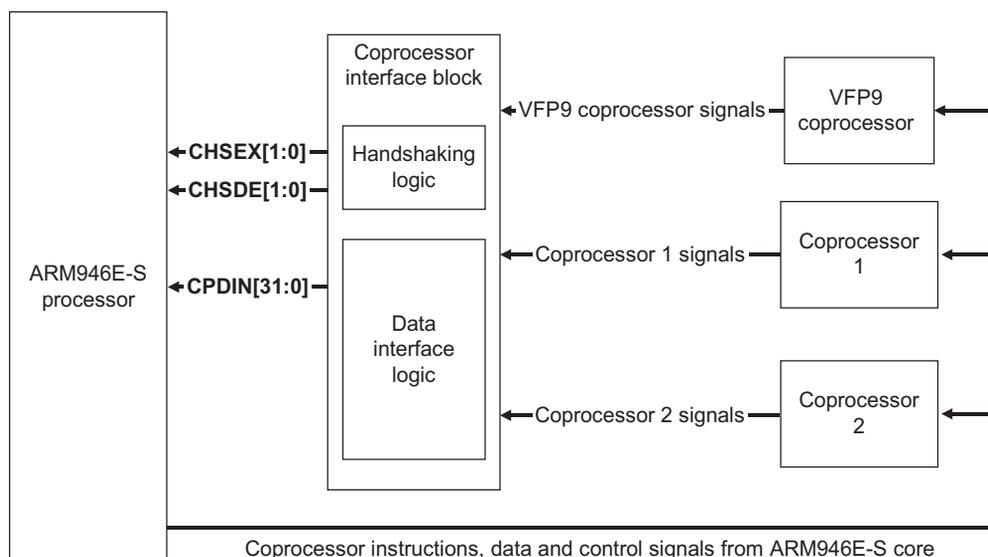
**Figure 7-2 Connecting multiple coprocessors**
