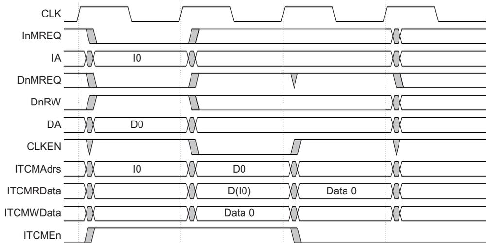
**Figure 5-7 Simultaneous instruction fetch and data write**
