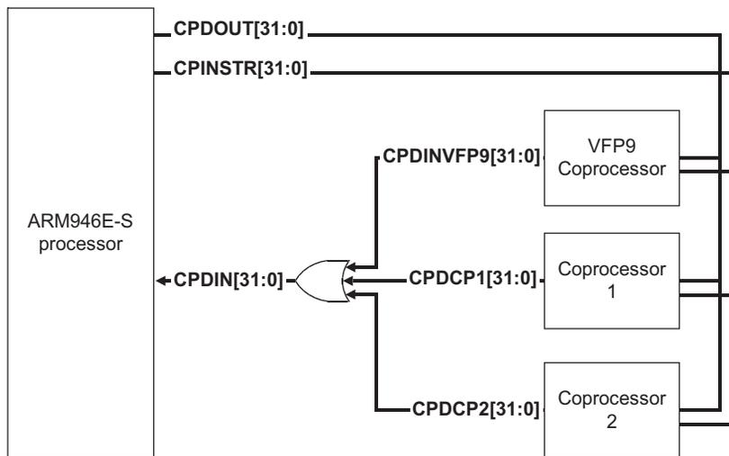
**Figure 7-4 Driving the coprocessors data buses to logic 0**
