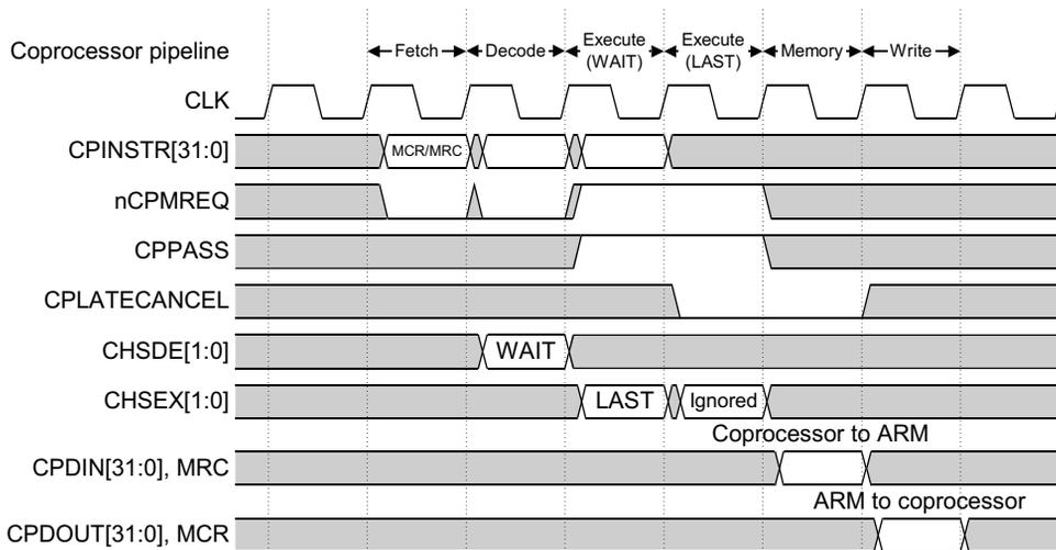
Figure 7-7 MCR/MRC transfer timing with busy-wait
