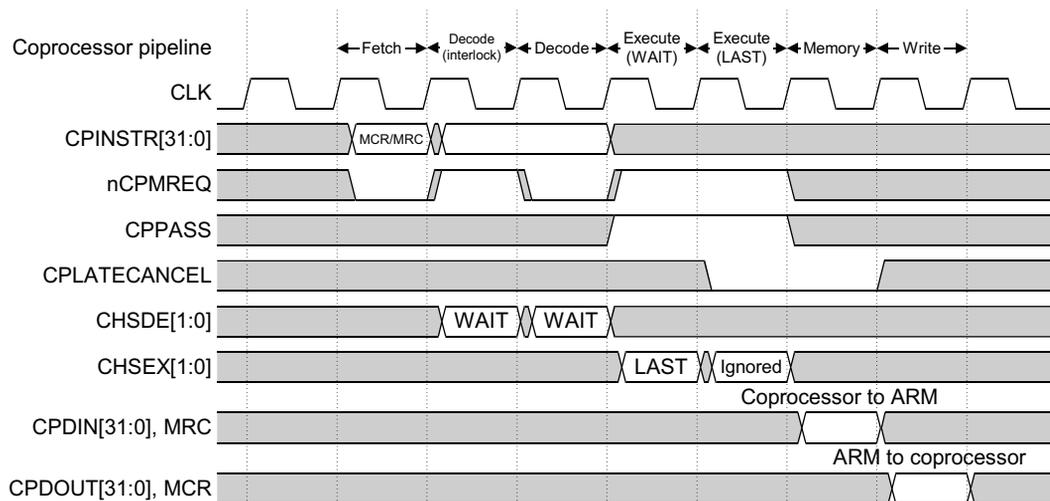
Figure 7-8 Interlocked MCR/MRC timing with busy-wait
