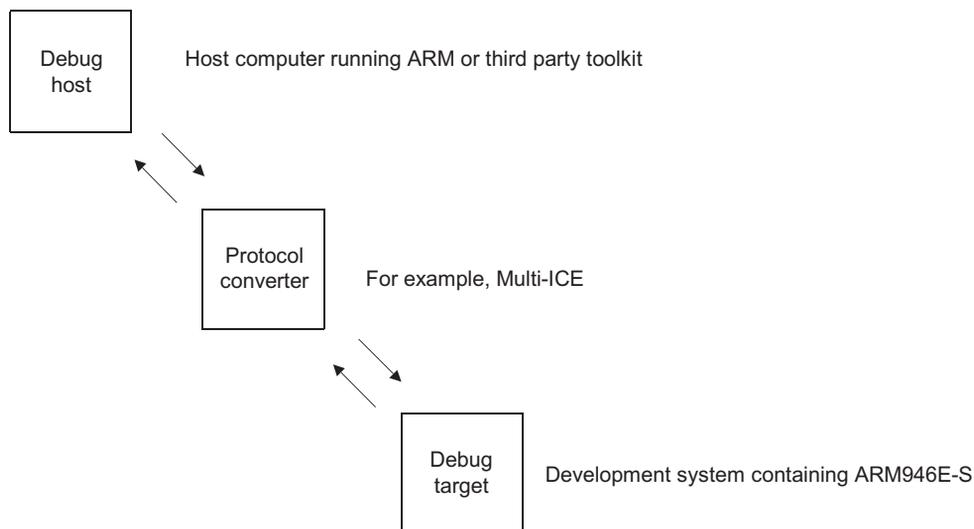
**Figure 9-2 Typical debug system**
