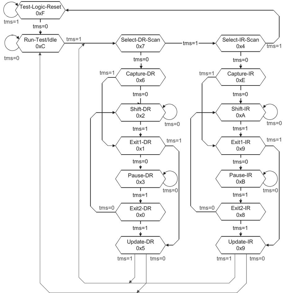
Figure 9-4 TAP controller state transitions<sup>1</sup>
