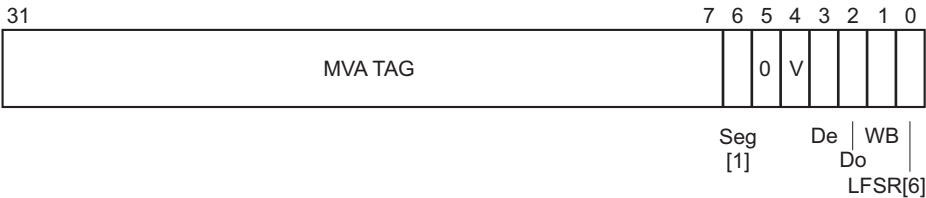
Figure B-7 Data format, CAM read
