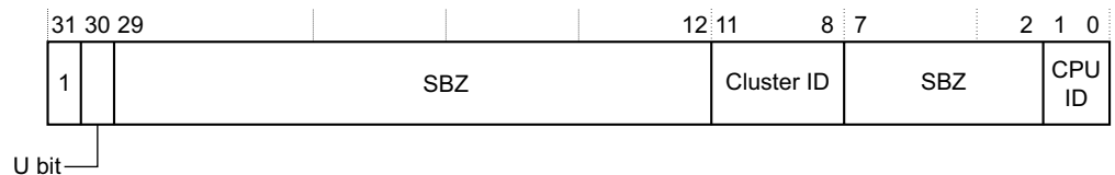
Figure 4-2 MPIDR bit assignments
