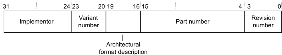
Figure 4-14 MIDR bit assignments
