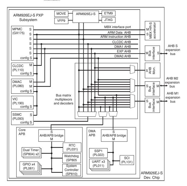
Figure 1-2 ARM926EJ-S Development Chip block diagram
