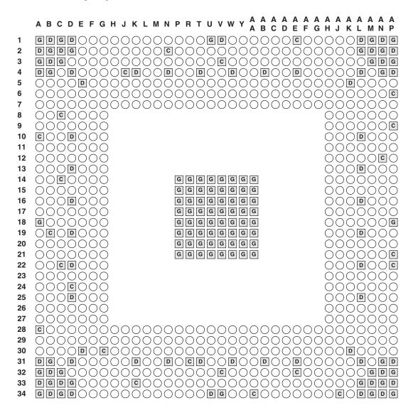
Figure B-1 BGA numbering, ball side view
