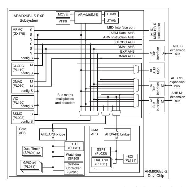
Figure 3-1 Bus matrix configuration
