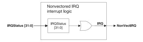
Figure 17-4 Nonvectored IRQ interrupt logic
