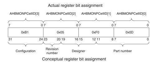
Figure 4-4 PrimeCell ID register
