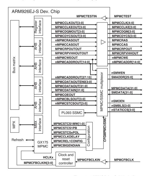
Figure 10-1 MPMC PrimeCell block diagram
