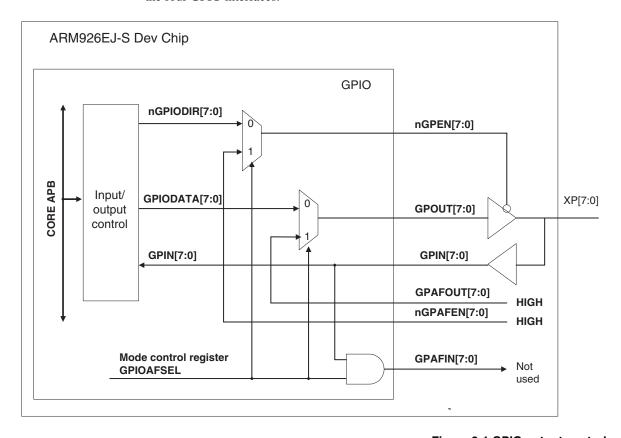
Figure 9-1 GPIO output control
