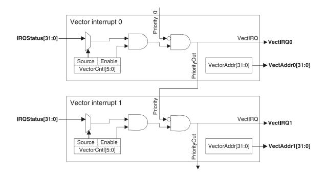
Figure 17-5 Vectored interrupt block
