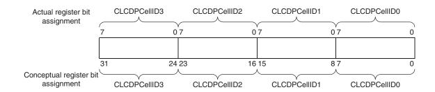
Figure 5-17 CLCDCPCellID0-3 Register bit assignments
