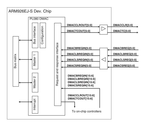
Figure 8-1 DMAC interface block diagram
