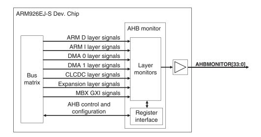
Figure 4-1 AHB monitor block diagram
