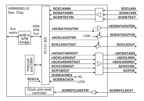
Figure 12-1 SCI block diagram
