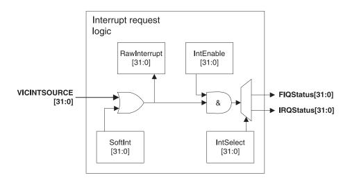
Figure 17-2 Interrupt request logic
