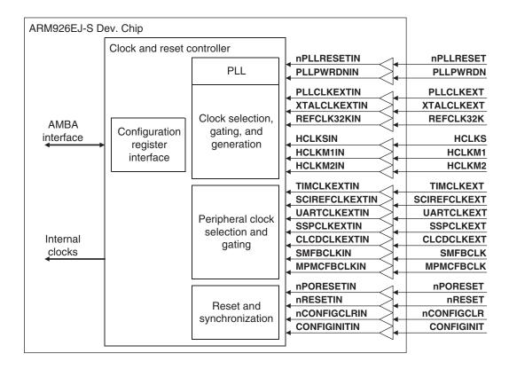
Figure 2-4 Clock and reset block diagram
