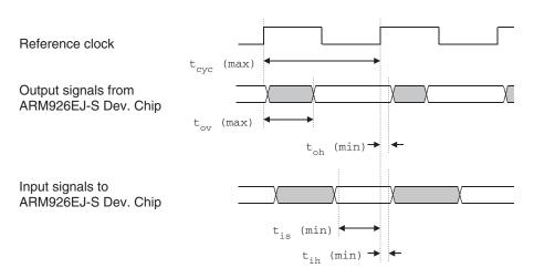
Figure C-1 AC timing example
