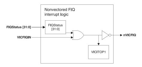
Figure 17-3 Nonvectored FIQ interrupt logic
