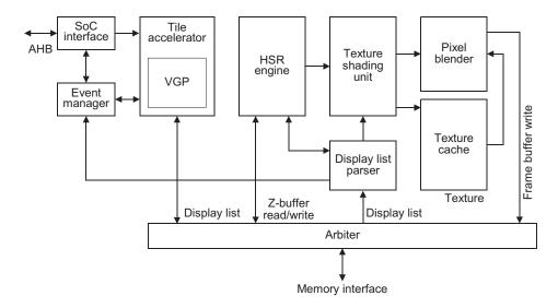
Figure 7-1 ARM MBX HR-S top level block diagram
