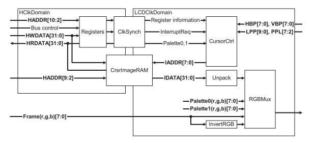
Figure 5-3 Hardware cursor block diagram
