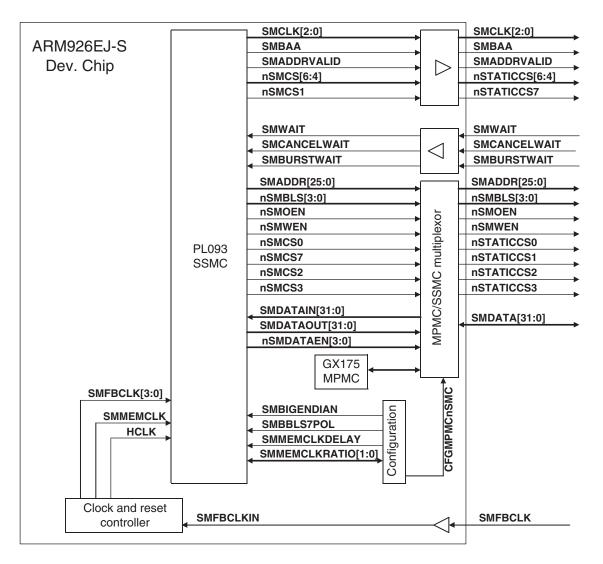
Figure 13-1 SSMC interface block diagram
