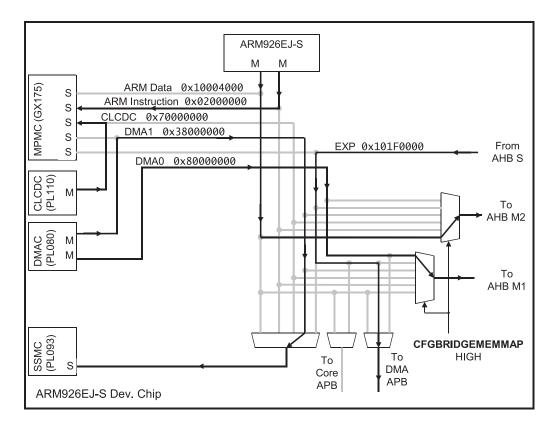
Figure 3-8 AHB M1 access determined by address range
