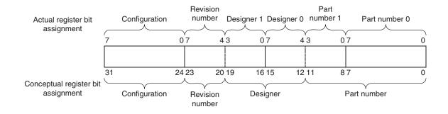
Figure 5-16 CLCDPeriphID0-3 Register bit assignments
