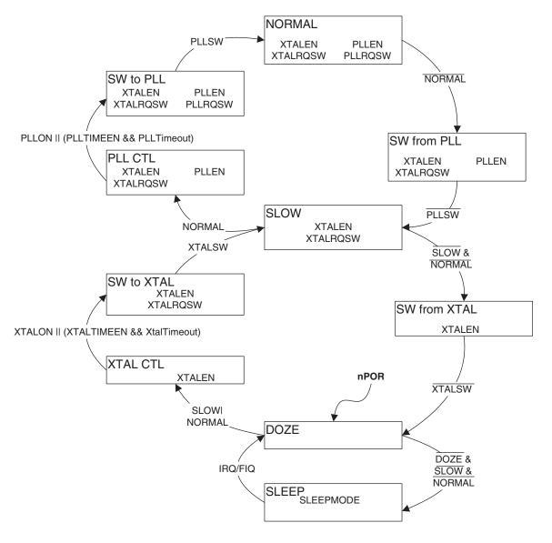
Figure 2-3 System mode control state machine
