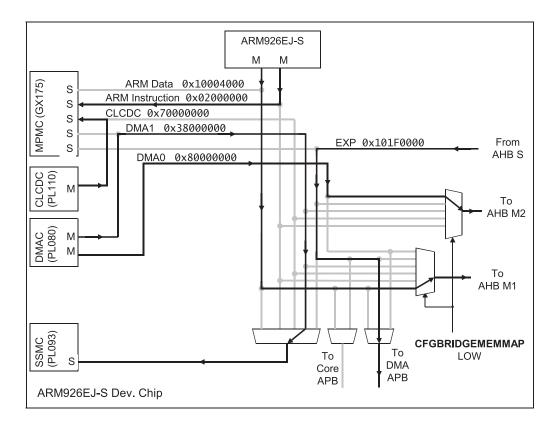
Figure 3-9 AHB M1 access determined by ARM D
