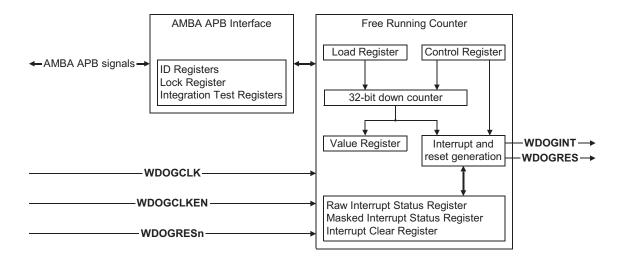
Figure 19-1 Simplified block diagram
