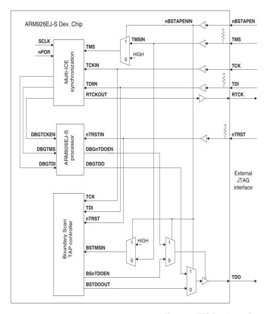
Figure 2-7 JTAG Test Access Port
