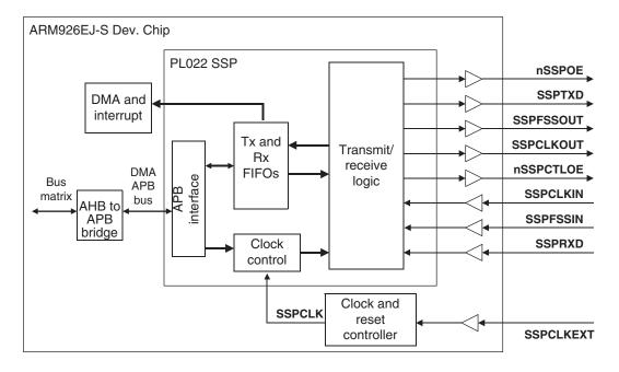
Figure 14-1 PrimeCell SSP block diagram
