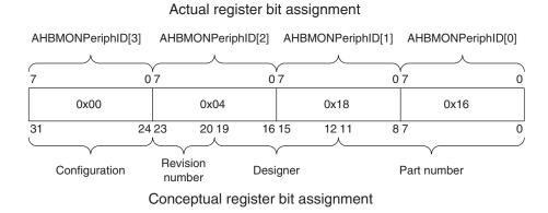
Figure 4-3 Peripheral ID register
