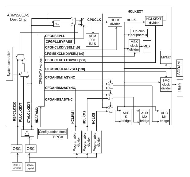
Figure 2-5 External clock signals and clock selection
