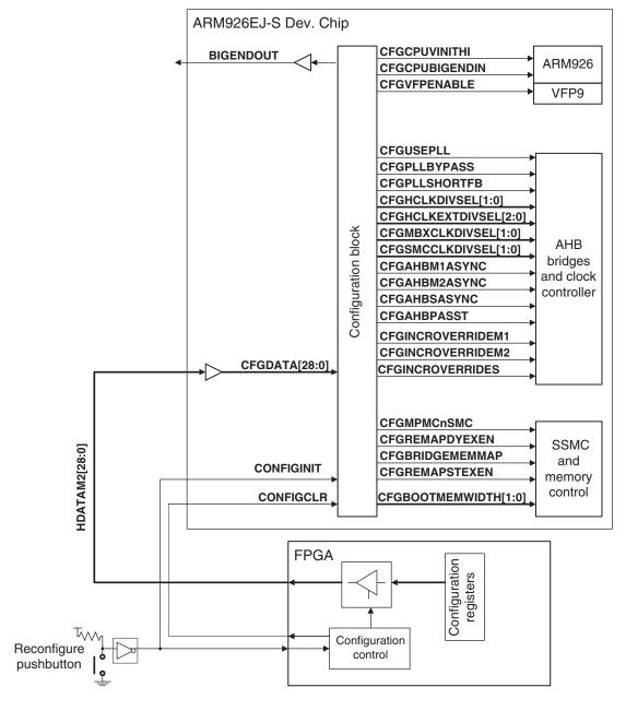
Figure 2-6 Power-on configuration block diagram
