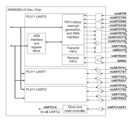
Figure 16-1 PrimeCell UART block diagram
