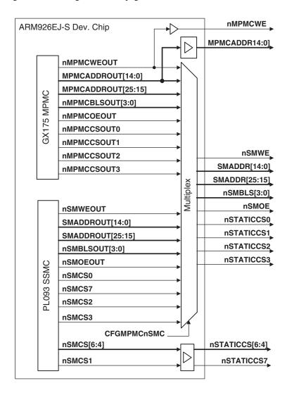
Figure 13-2 Address and control multiplexor
