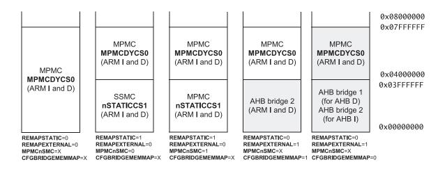
Figure 3-13 Supported address remap functionality for ARM D AHB
