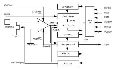
Figure 3-1 Joystick interface block diagram
