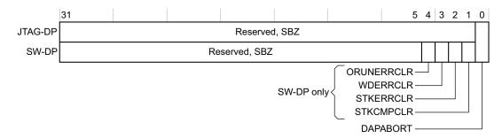
Figure 9-21 Abort Register bit assignments
