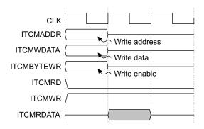
Figure 10-1 ITCM write signal timings
