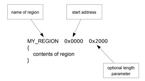
Figure 6-6 Scatter-loading description syntax
