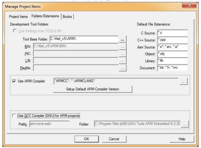
Figure 1-3 Accessing the Arm Compiler version from Keil  $\mu$ Vision
