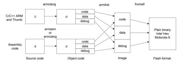
Figure 1-1 A typical tool usage flow diagram
