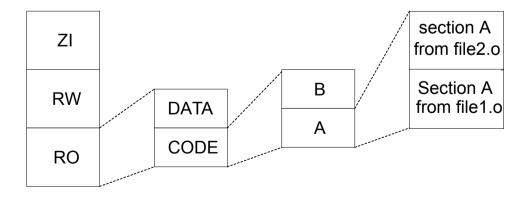
Figure 6-3 Linker placement rules
