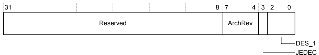
Figure 4-33 GITS_PIDR2 bit assignments
