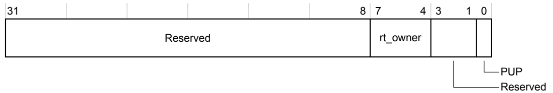
Figure 4-7 GICD_DCHIPR bit assignments
