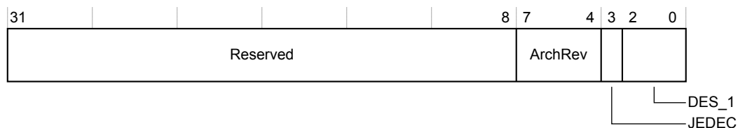
Figure 4-14 GICD_PIDR2 bit assignments
