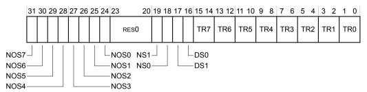
Figure B1-54 PRRR bit assignments
