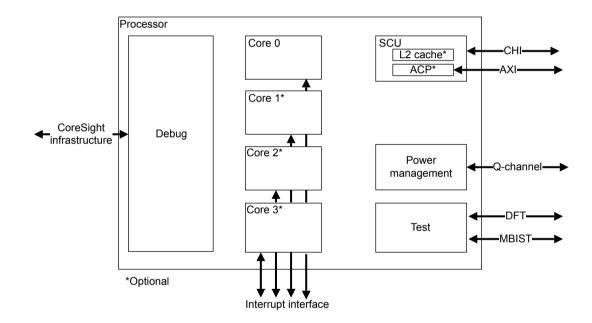
Figure A1-1 Example processor configuration
