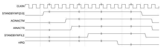
Figure A4-3 L2 Wait For Interrupt timing
