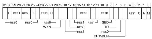
Figure B1-23 HSCTLR bit assignments
