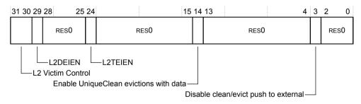
Figure B1-45 L2ACTLR bit assignments
