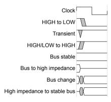
Figure 1 Key to timing diagram conventions
