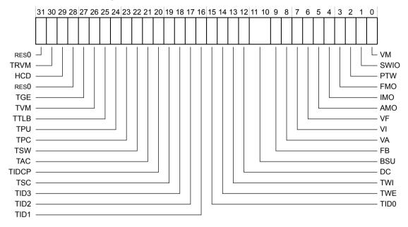
Figure B1-17 HCR bit assignments
