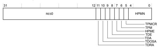
Figure B1-19 HDCR bit assignments
