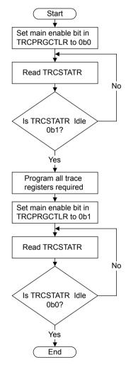
Figure C3-2 Programming ETM trace unit registers
