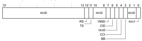
Figure C10-3 TRCCONFIGR bit assignments
