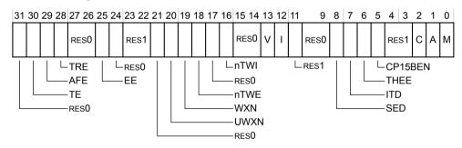
Figure B1-58 SCTLR bit assignments
