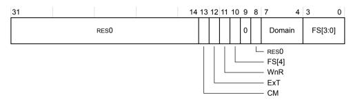
Figure B1-13 DFSR bit assignments for Short-descriptor translation table format
