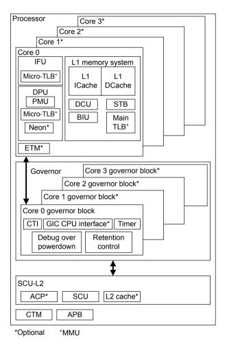
Figure A2-1 Cortex-A32 processor block diagram
