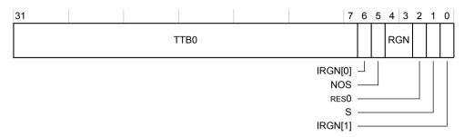
Figure B1-63 TTBR0 bit assignments, TTBCR.EAE is 0
