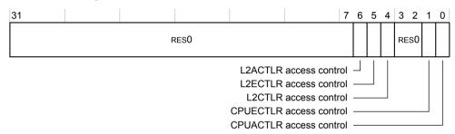
Figure B1-15 HACTLR bit assignments
