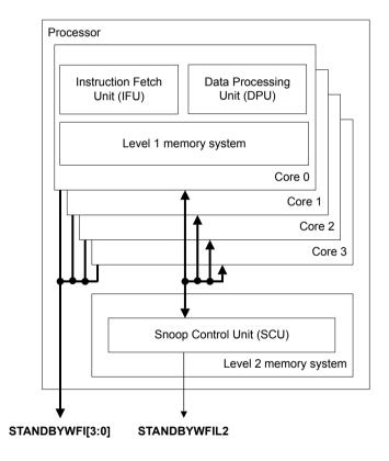
Figure A4-4 STANDBYWFI[3:0] and STANDBYWFIL2 signals
