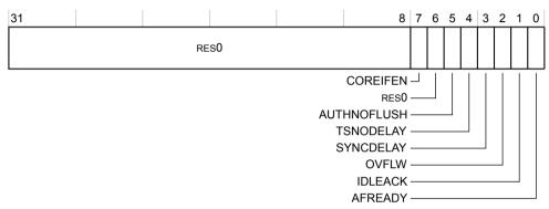
Figure C10-5 TRCAUXCTLR bit assignments
