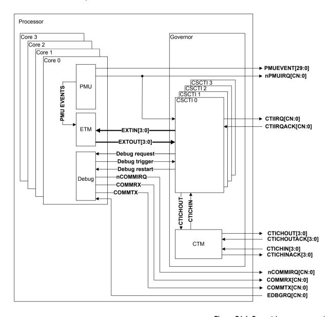
Figure C4-1 Cross-trigger components
