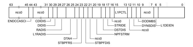
Figure B1-6 CPUACTLR bit assignments
