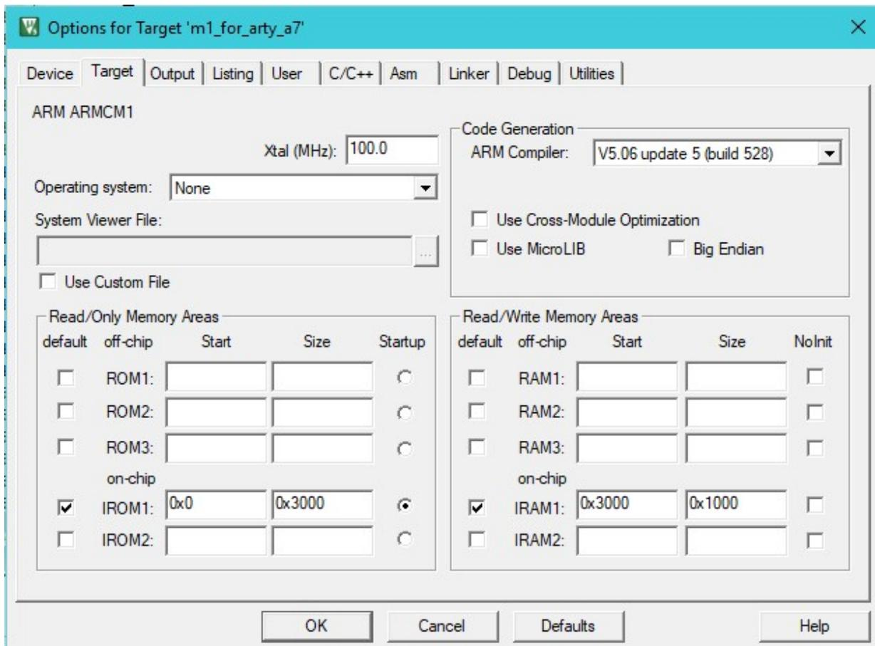
Figure 3-5 Example Keil configuration
