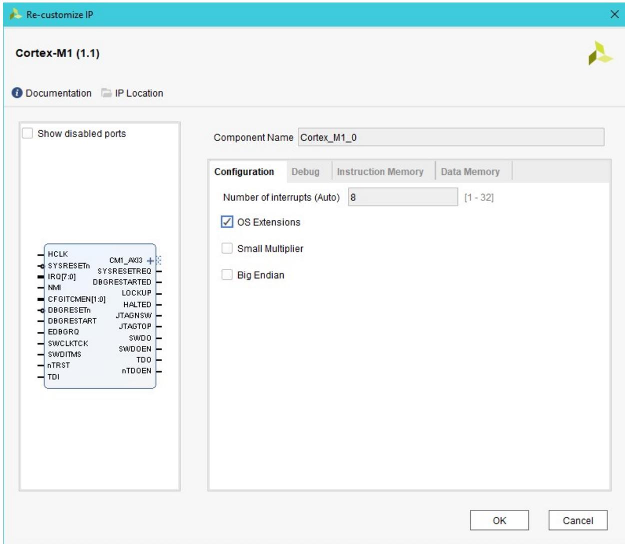
**Figure 3-1 Configuration tab**
