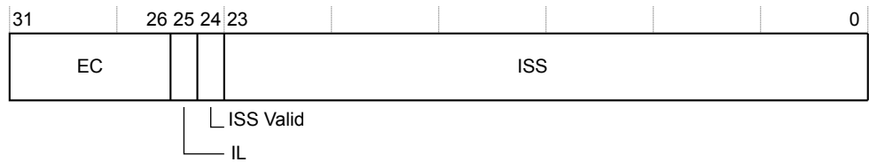
Figure 4-53 ESR_EL1 bit assignments
