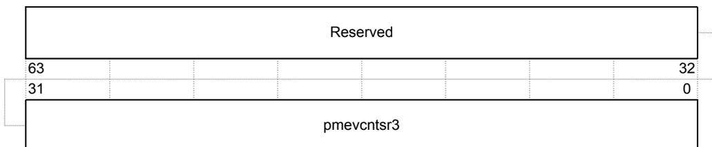
**Figure 3-112 pmevcntr3 register bit assignments**
