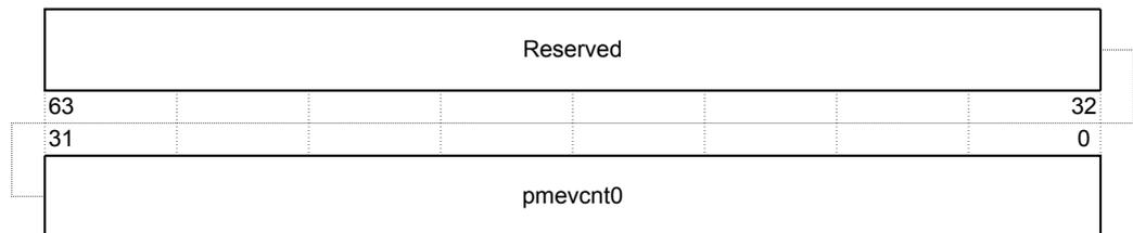
**Figure 3-100 pmevcnt0 register bit assignments**
