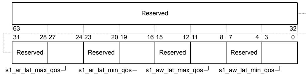
**Figure 3-134 s1\_qos\_lat\_range register bit assignments**
